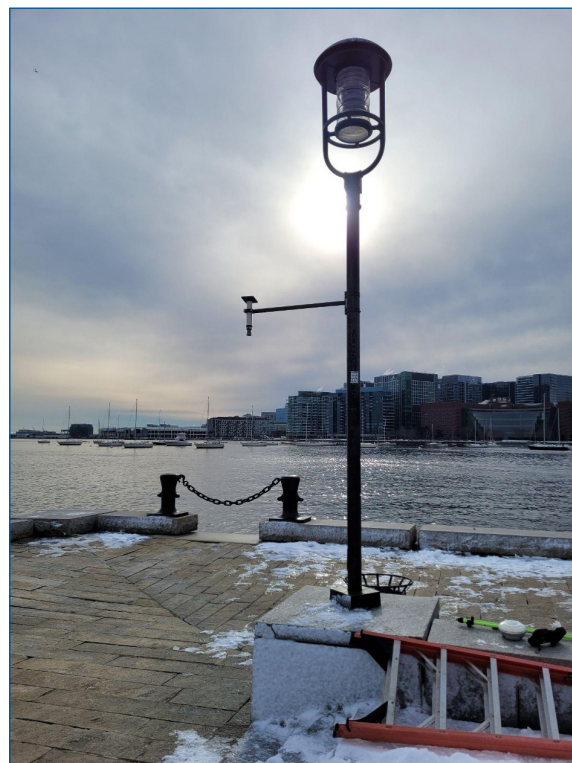
Left: Hohonu water level sensor mounted overland for inundation event alerts in Boston, MA
